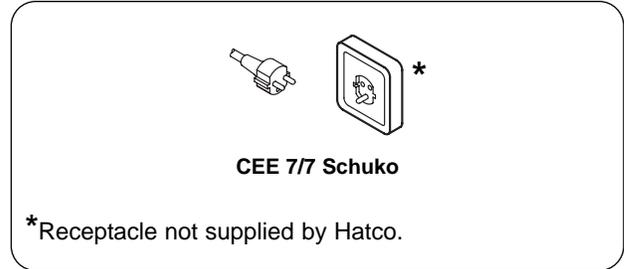
Figure 2. Plug Configurations
